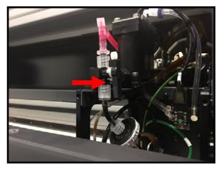
The other manual 3 way valve is located at the front of the print carriage in the bottom left corner.
