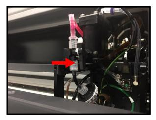
Move the bottom manual 3 way valve so it is in the 9:00 (9 o'Clock) position. This will let the ink flow through the purge line.
