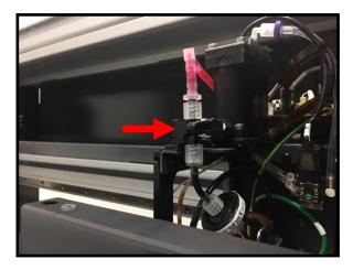
Move the bottom manual 3 way valve so it is in the 9:00 (9 o'Clock) position. This will let the pink flushing solution flow through the purge line and evacuate the ink that is in place.
